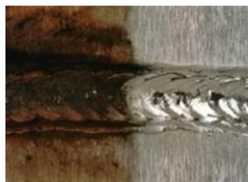
***The newer method of using nitric followed by a non-caustic alkaline cleaner*** is now widely used in the brewing industry as one of the best ways to keep your metal clean **AND** passivated.
